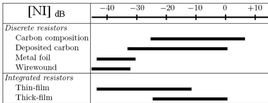
Fig.2: Average noise indexes of commercial resistors [2, p.168].
