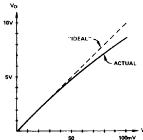
Fig.4: Nonlinear transfer functions of audio amplifier [4, p.3].
